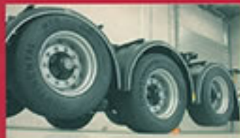
Lift axles are possible on types CT-53-04D 3x, CT-53-05D and CT-60-05D 4x.
